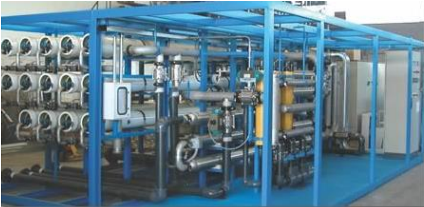
EAST MEDITERRANIAN UNIVERSITY AND MAGOSA MUNICIPALITY Sea Water Treatment System for Drinking and Usage Water Production Reverse Osmosis System with Prefiltration Group 1.000 m 3 /day
