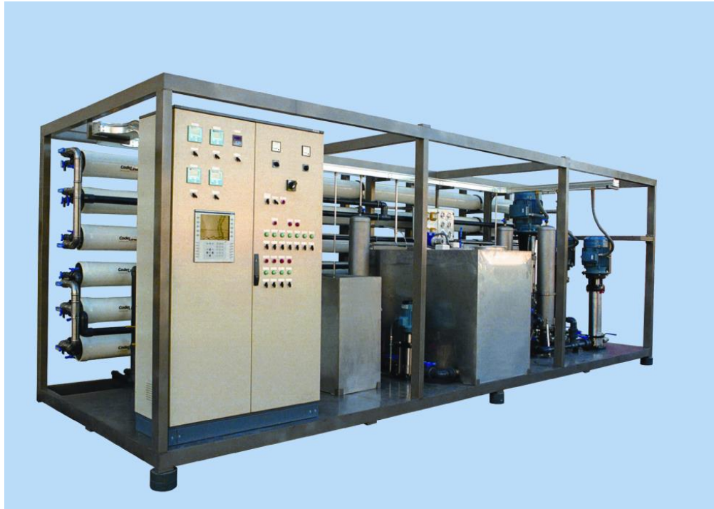
TURKEY SUGAR FACTORIES Steam Boilers Feeding & Drinking and Usage Water Production Reverse Osmosis System with Prefiltration Group 30 m 3 /hour
